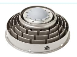
The GNSS-750 revolutionary choke ring antenna supports GPS, GL0NASS, Galileo, and COMPASS satellite signals. Its unique 3-D conic form factor enhances low-elevation tracking and provides excellent multipath mitigation. Cast with aluminum alloy, the GNSS-750 can withstand severe environmental conditions, making it ideal for reference stations, monitoring, seismic stations, scientific and other applications requiring a robust high-performance antenna.
